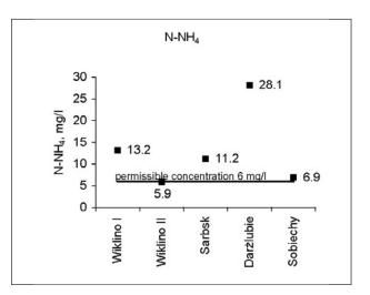
Fig. 5. Average concentration of ammonia nitrogen and total nitrogen in effluent in hybrid system.
