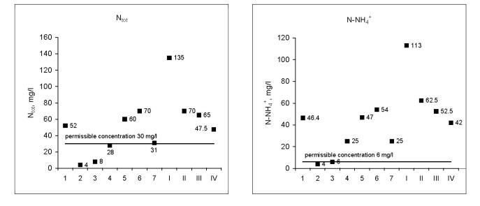
Fig. 1. Average concentration of ammonia nitrogen and total nitrogen in effluent in individual HF-CWs.
