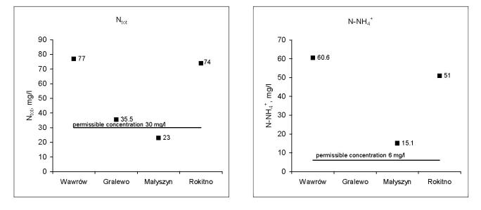
Fig. 3. Average concentration of ammonia nitrogen and total nitrogen in the effluent in local HF-CWs near Gorzów, Poland.
