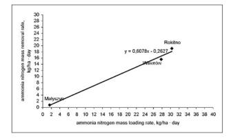
Fig. 4a. Ammonia nitrogen mass loading and removal rates in local HF-CWs near Gorzów, Poland.
