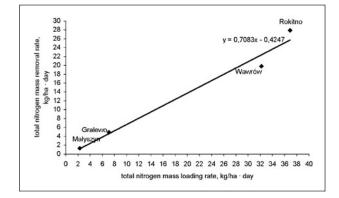
Fig. 4b. Total nitrogen mass loading and removal rates in local HF-CWs near Gorzów, Poland.
