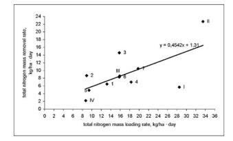
Fig. 2b. Total nitrogen mass loading and removal rates in HF-CW household system.
